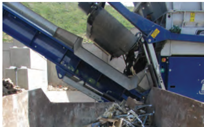
Overband Magnet - fitted to discharge conveyor to extract ferrous metal
