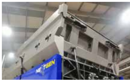
Hydraulic Raise / Lower Hopper Extensions
